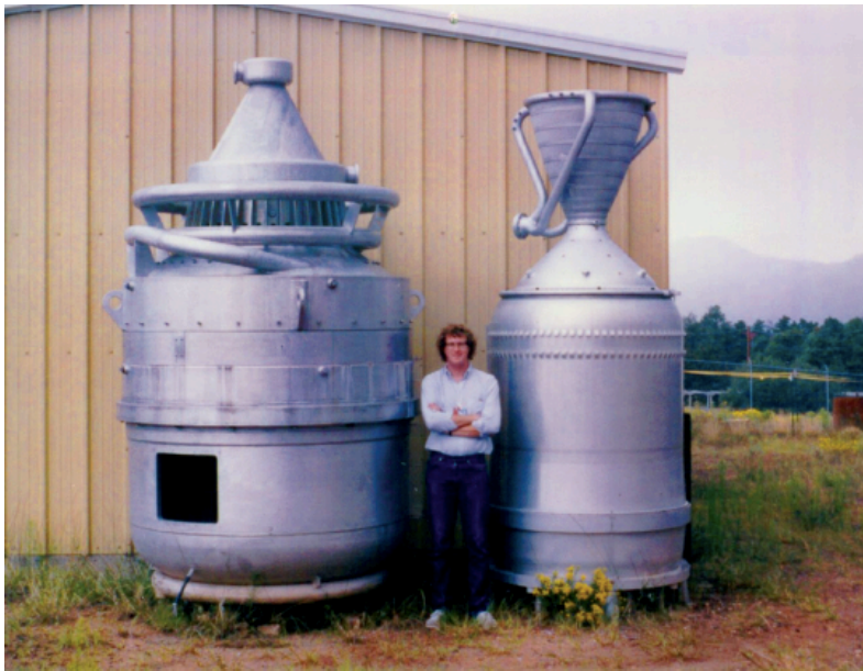
Figure 3-2. Nuclear Rocket Test Equipment from LANL's Rover Program. The equipment from the first phase (Kiwi) is on the left. Equipment from the second phase (Phoebus) is on the right.
