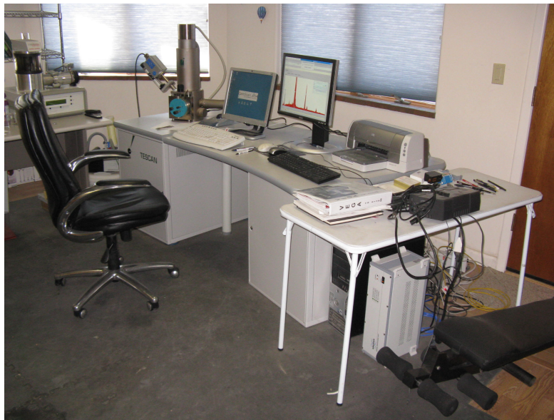
Figure 7-2. Scanning Electron Microscope (SEM) with Energy-Dispersive X-Ray (EDX) Spectroscopy Capability. The SEM is the tall vertical cylinder. The EDX is the instrument just to the left of the SEM.
