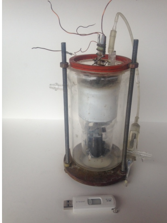
Figure 7-5. Calorimeter Used by Dr. Storms at LANL for Early LENR Studies at Los Alamos National Lab. Note the electrolytic cell inside the cell near the bottom. Thumb drive is 2.75 in long. Photo taken April 2016.
